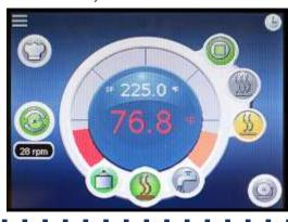
Above is SAMPLE Screen display. In this example, the Heat is set to 225F. 'Cook To' temperature can be set to fit your product's optimum temperature.
